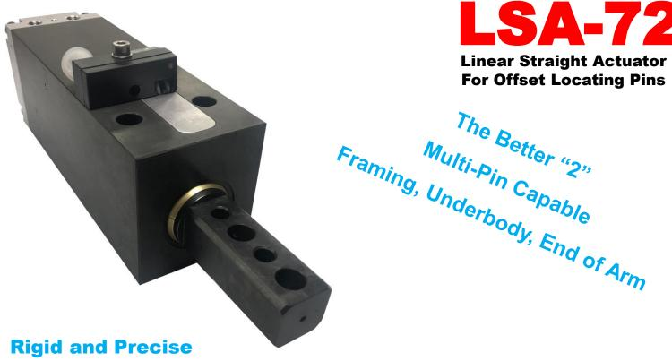
The LSA-72 uses a ceramic bearing system that provides absolute rigidity with a patented slider for anti-rotation This technology combined with CNC precision results in RapStop™; a system integral to every unit. RapStop™ replaces external stops and rap couplings while it maintains Z-Axis accuracy to ± 0.050 mm. Tested with over 3,000,000 cycles and a 24kg load, the LSA-72 demonstrated less deflection than any commercially available locating pin and complies with every auto maker's requirements.
